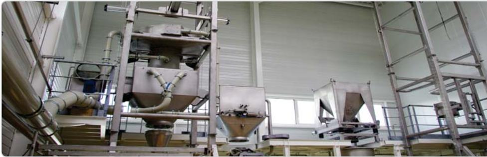
Unloading solution: FIBC, bag, container (semi-automatic, containment, ergonomic, ATEX dust collector, loss-in-weight stations, big bag massing paddles)
