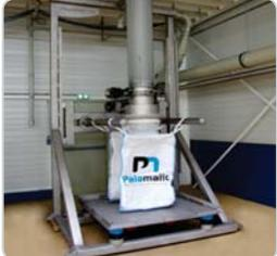
Big bag filling station: vibrating table and weighing
