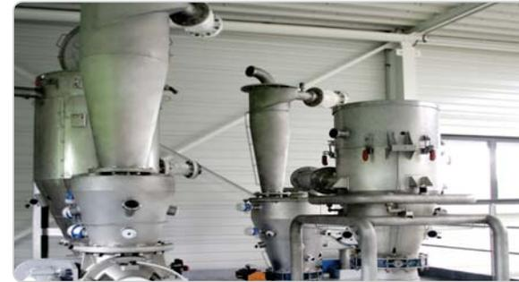
Pneumatic conveying equipment: pressure, vacuum, dilute or dense phase
