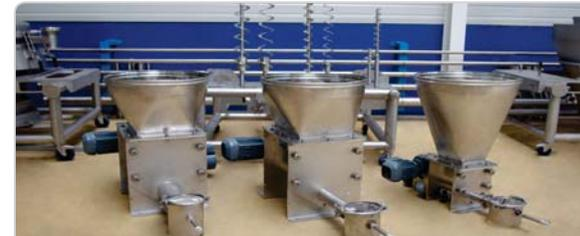
Feeders: 3 models (D11, D12, D13) with capacity from 5 to 3,500 liters with weight or volumetric feeding
