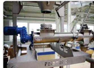
Screw conveyor: easyclean and adjustable slope
